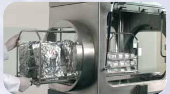
Sliding trolley for ease of load transfer
